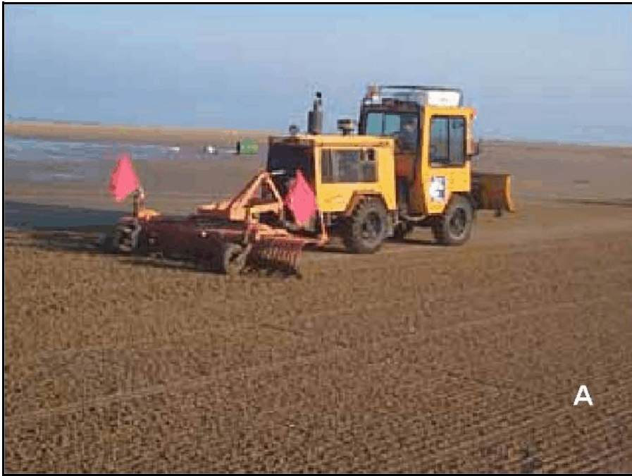
Figure 4a: Beach raker at Sauble Beach. Vehicle owned and operated by the municipality. Typically the raking is done 3 or 4 times a week in the summer season.
